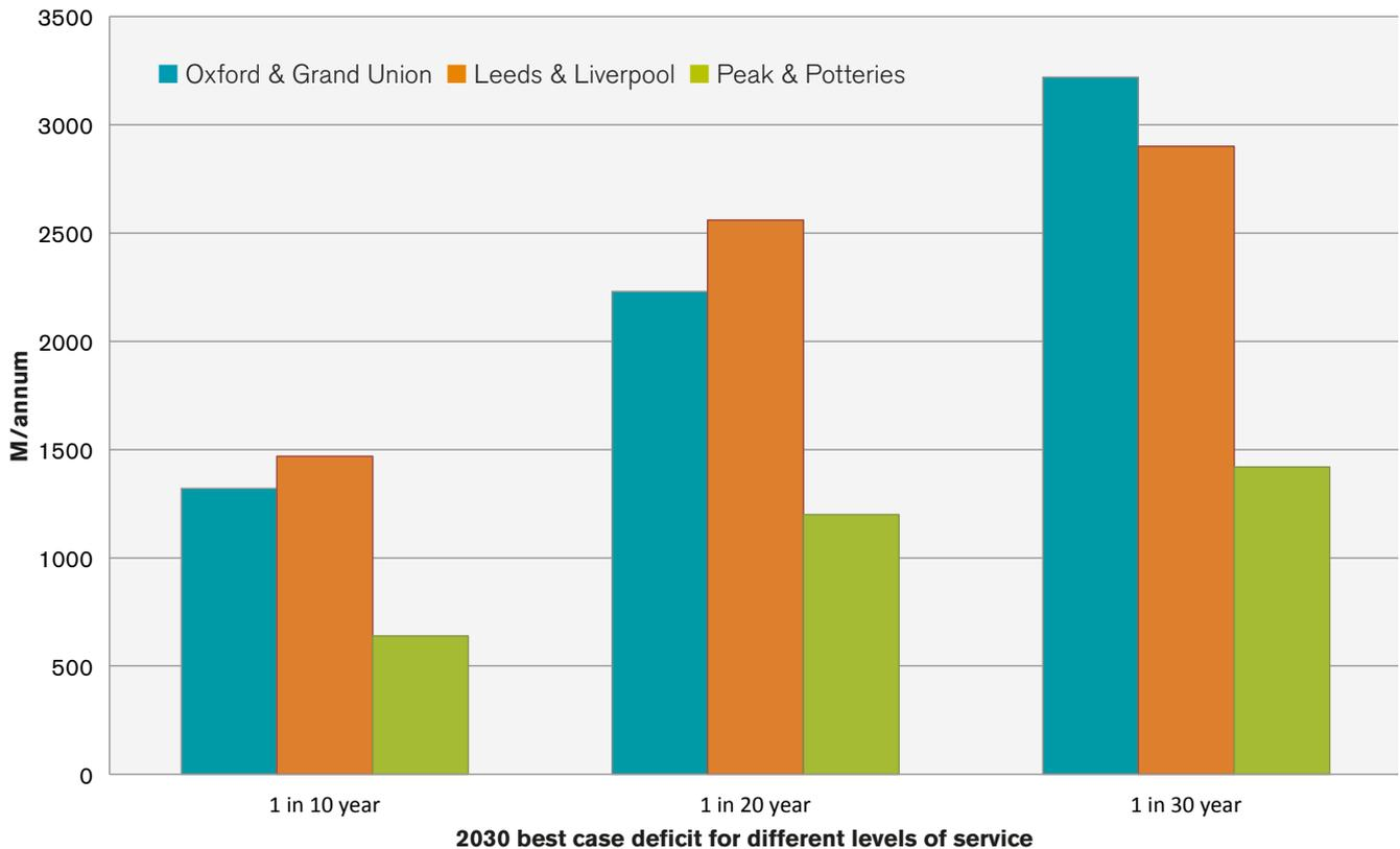
**Figure 3: Best case projected deficit (M) for the three levels of service**
