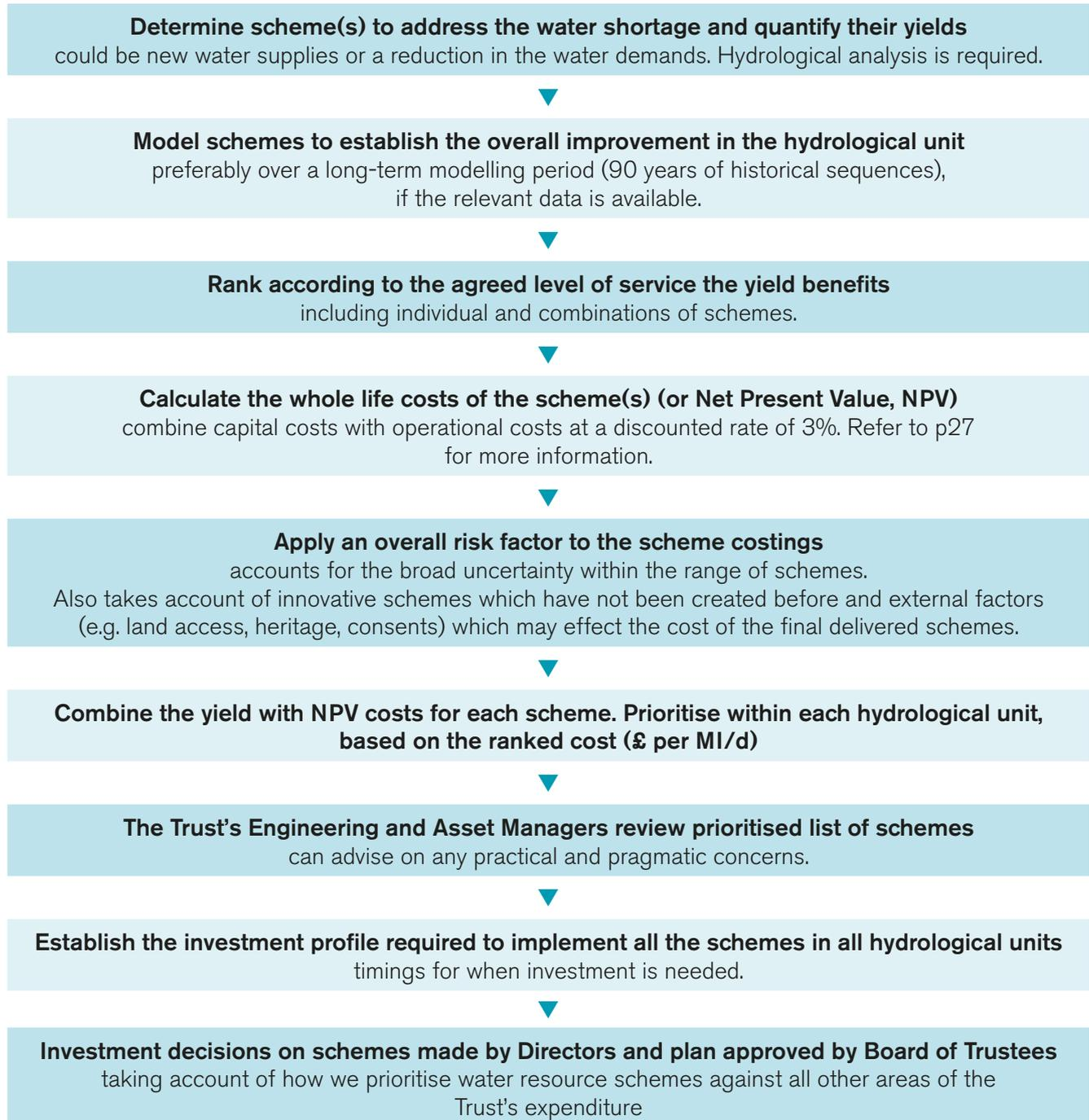
Figure 5: Flow diagram for deciding on water resources improvements
