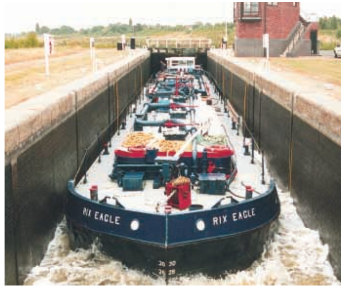
'Rix Eagle' loaded with 500 tonnes of gas oil from Immingham seen here passing through Lemonroyd Lock on the Aire and Calder Navigation en route to Bayford Fuels depot at Fleet, near Leeds. Petroleum products and other liquid bulks are particularly suited to waterway transport because they are easy to pump in and out of barges directly to or from waterside tank storage facilities. Waterborne freight is a safe and reliable mode of transport for such hazardous cargoes. This barge is saving around 42 road tanker trips between Immingham and Leeds: clearly a more environmentally sustainable means of freight transport. This traffic is another example of Government assistance in the form of a Freight Facilities Grant (to Bayford Fuels) making a contribution to modal shift from road to water. (Source: Mike Brown)
