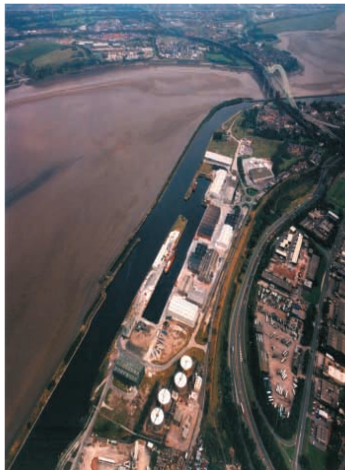
The Manchester Ship Canal extends 35 miles from Eastham on the River Mersey to Manchester. The Canal can accommodate seagoing ships of up to 8,000 tonne cargo capacity in its upper reaches. The lower reaches of the Canal accommodate much larger vessels that serve the petroleum and chemical industries along its banks at Stanlow and Ellesmere Port. In 2002 the Canal handled 6.7 million tonnes of cargo. Runcorn Docks is a busy small port on the Canal specialising in handling bulk commodities for the potteries amongst other industries. In 2002 it handled 350,000 tonnes of minerals, sands and fertilizer. Runcorn is a good example of the type of small port that can make a large contribution to the sustainable transport agenda for a local hinterland. The planning system needs to ensure the continuation of facilities of this kind by taking positive steps to encourage and facilitate appropriate industrial location. (Source: Manchester Ship Canal Company)
